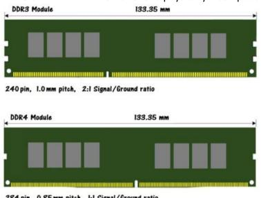
284 pin. 0.85 mm pitch. 1:1 Signal/Ground ratio
