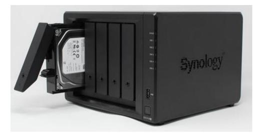
A NAS can have multiple bays (2,4,6,8 common) containing high capacity disk drives.
